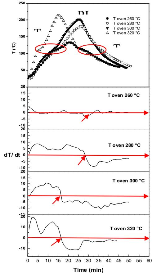
**Figure 1.** Internal air temperature (IAT) profiles and their derivatives as a function of time for LMDPE at different oven temperature and total cycle time. ■: 320 °C, 49 min; •: 300 °C, 53 min; ▲: 280 °C, 55 min, and ◆: 260 °C, 49 min.
