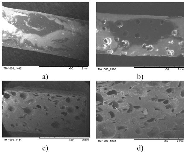
**Figure 4.** Micrographs of the final LMDPE morphology with different ACA content: a) 0%, b) 0.25%, c) 0.50%, d) 1.0% wt.
