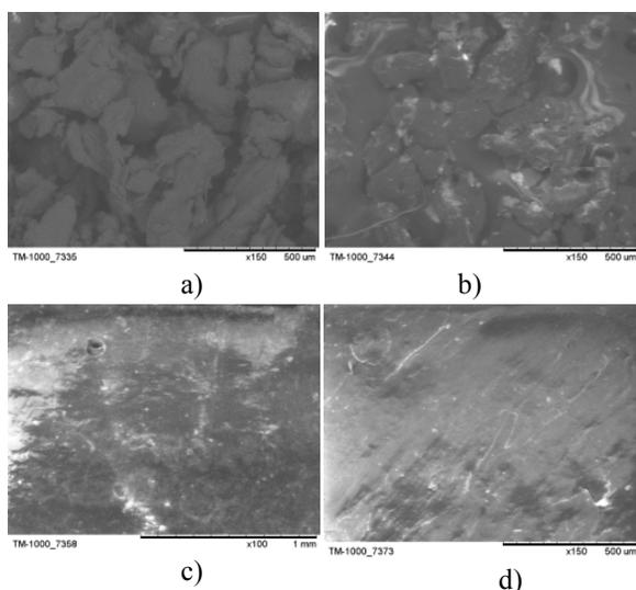
**Figure 2.** Micrographs of neat LMDPE taken at different stages of the rotomolding cycle for an oven temperature of 280 °C: a) 5 min, b) 10 min, c) 15 min, and d) 20 min.
