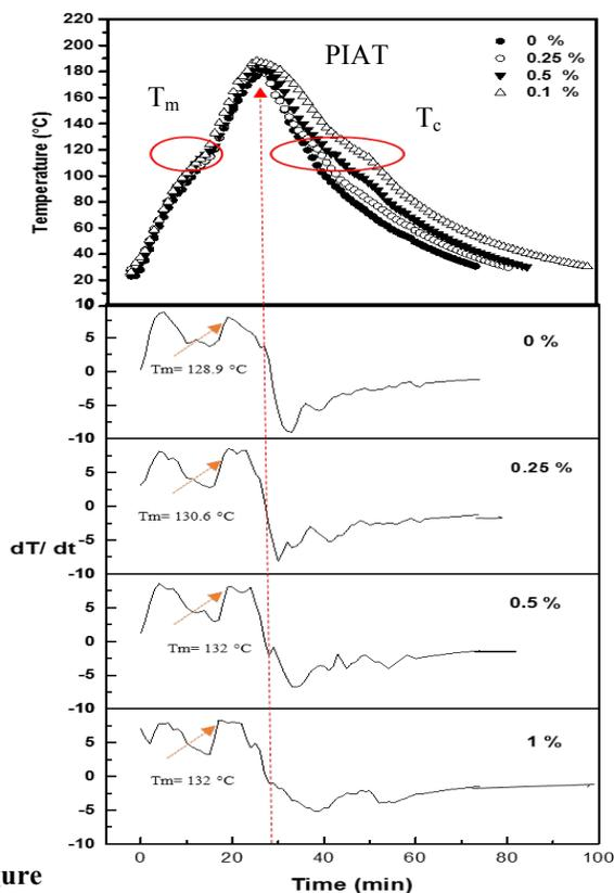
**Figure 3.** Internal air temperature (IAT) and derivatives as a function of time for unfoamed and foamed LMDPE at different ACA concentration.
